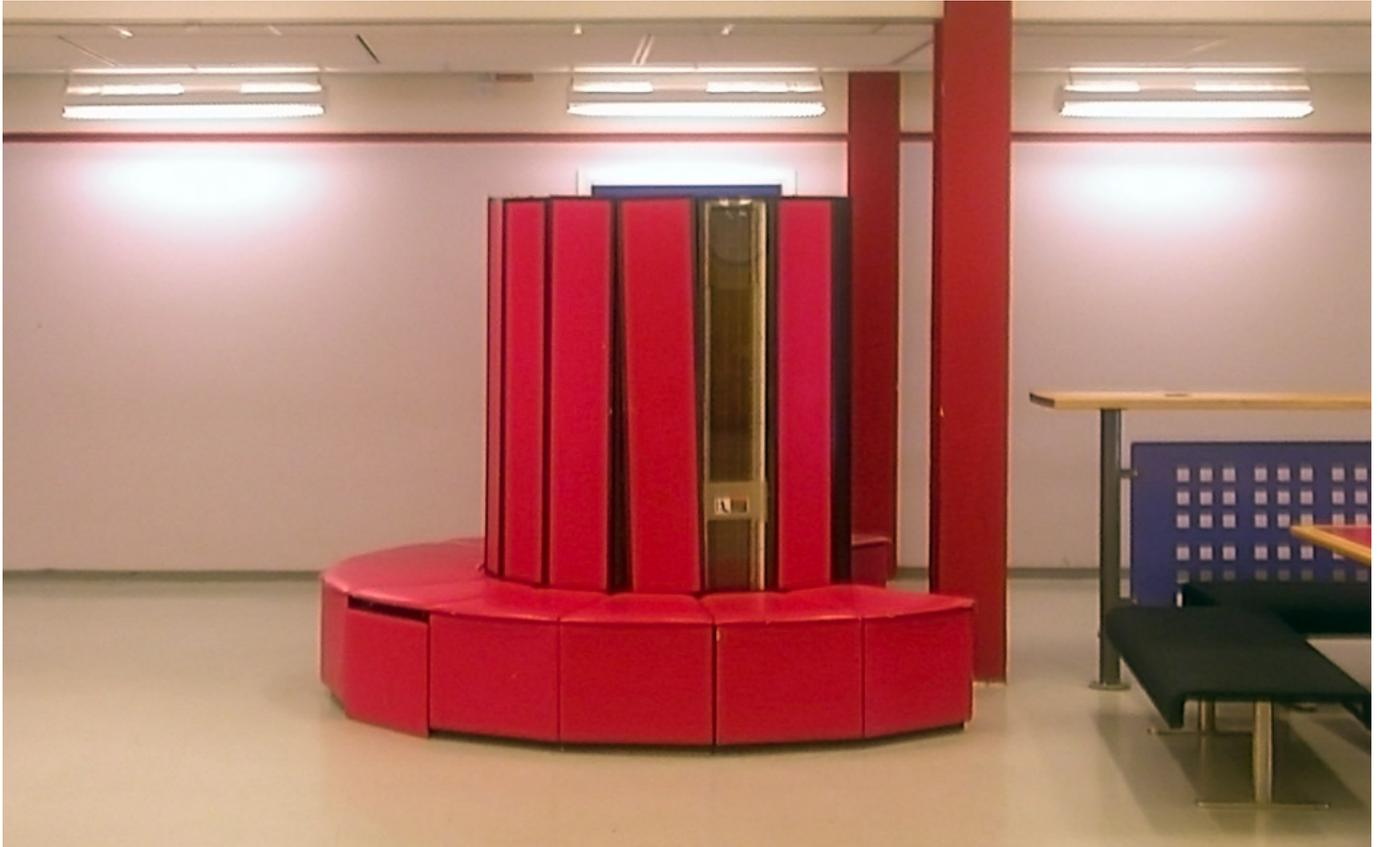
The fact that they packed four times as much HW into the same physical size meant that they had to use significantly higher integration. It also meant that the distance between key components got shorter due to the denser setup. These two factors resulted in a modestly higher clock rate of 105MHz, up from the original 80 of the Cray-1s. It's not clear to me from the documentation, but I would expect slightly higher latencies for far-away parts of the system, like the memory.
